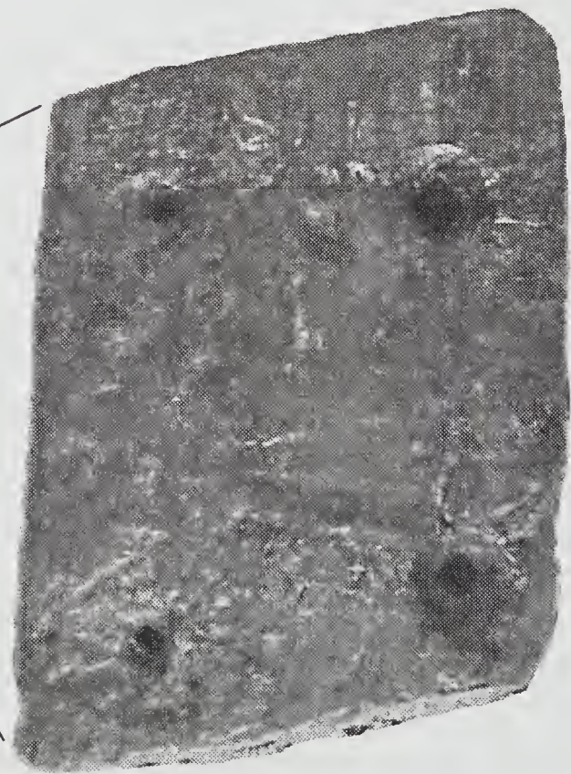
Figure 3. Bottom Planks— Numbers 437 and 493. Plank 437 exhibits a simple repair or "Dutchman"; Plank 493, a single repair (see enlarged detail) and the remains of a second near one end. Notice the typical fastening pattern of alternating treenail-spike, spike-treenail, etc.
