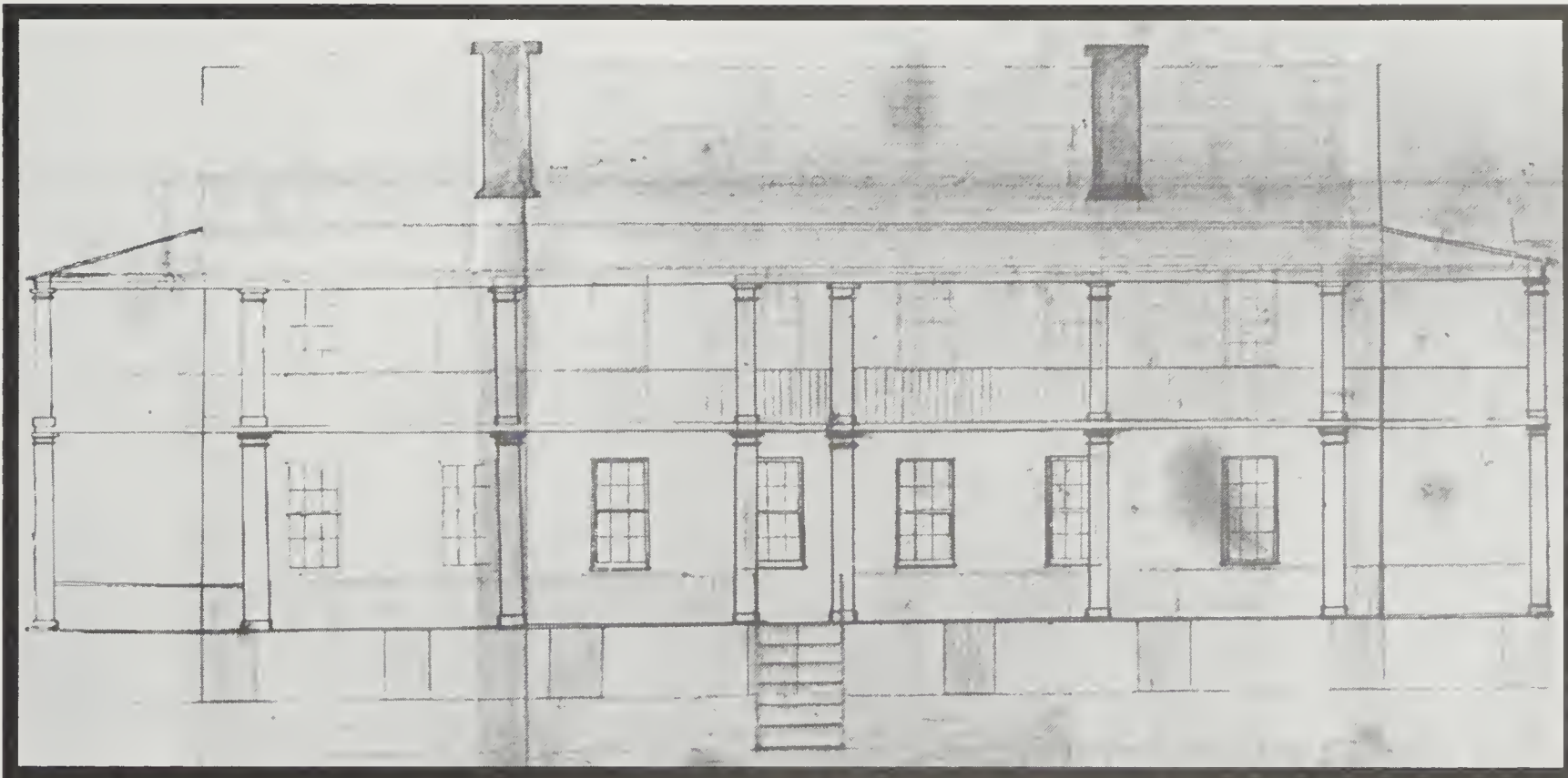
Side elevation of plan. Note the substantial piers supporting the structure which protected the lower floor from sea water (a frequent visitor to buildings on the island during storms) as well as the columned “piazzas” (porches).
