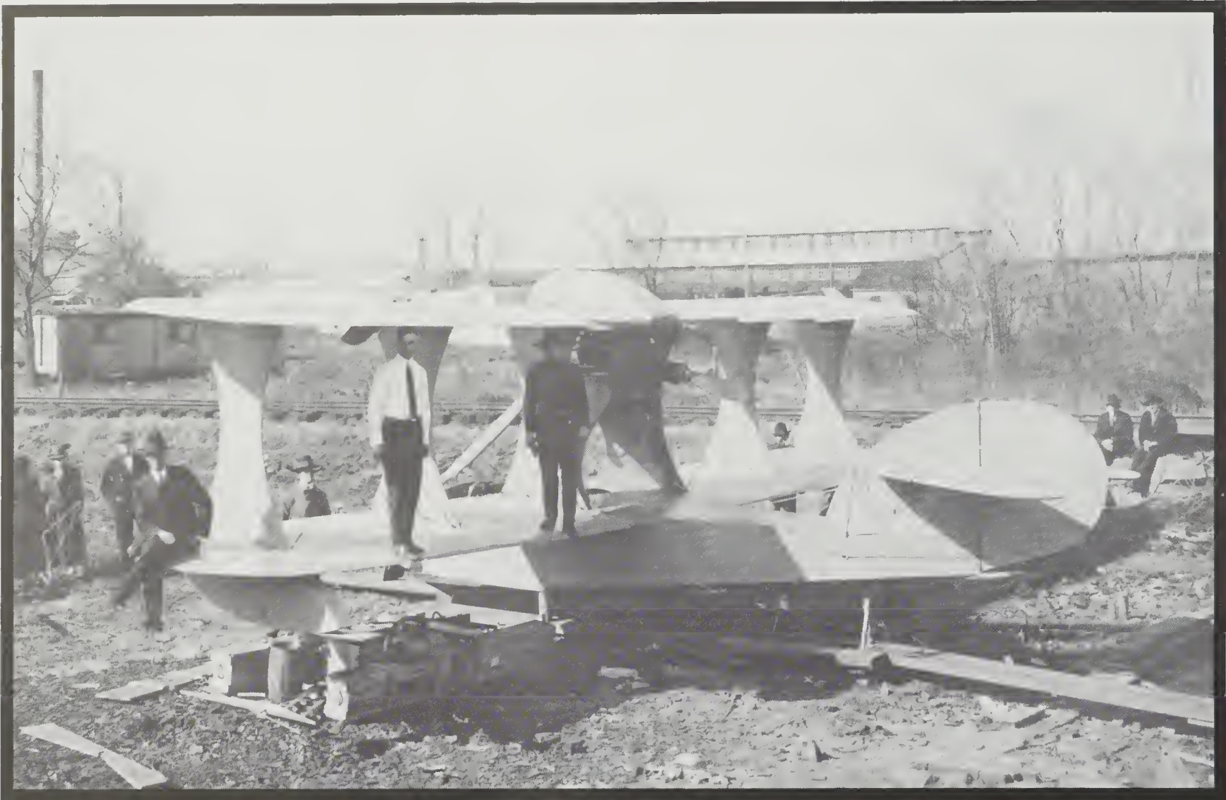
Atwood-modified Curtiss Model F flying boat ca. 1918 showing four sets of flying wires and demonstrating strength of wing covering material. Atwood is standing on trailing edge in the white shirt and tie. (Peter M. Bowers Collection)
